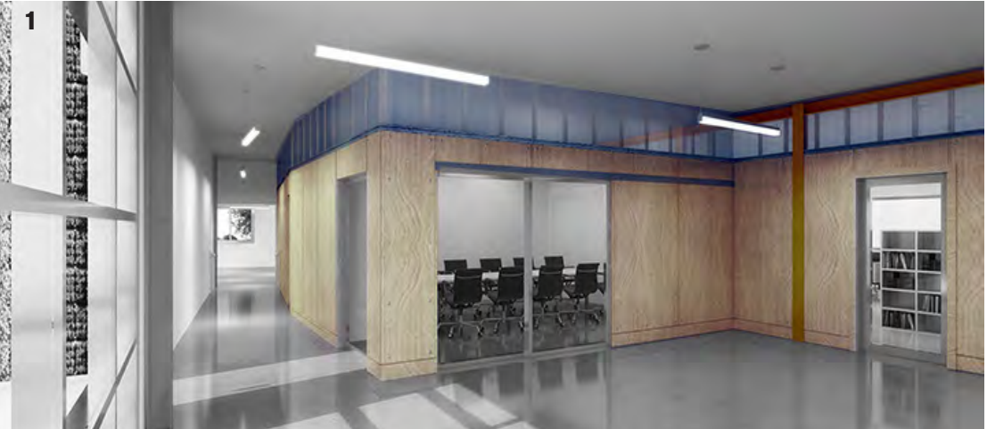
An 8'-6" plywood datum organizes the tenant spaces while translucent polygal clerestories transmit borrowed daylight, preserve openness, and reconcile varying ceiling heights.
